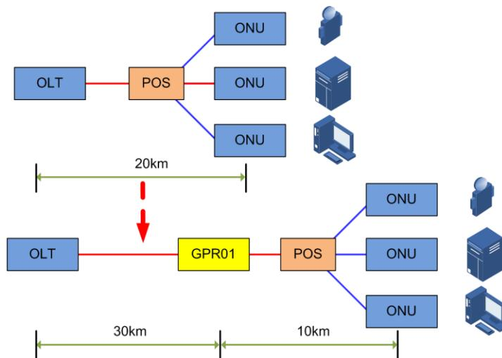
2. It is deployed between the OLT and optical splitter to increase optical splitting ratio, which can resolve the optical splitting ratio limit problem due to inadequate optical budget.
